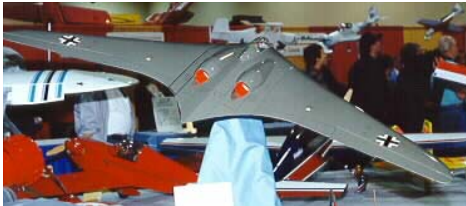
Keith Shaw's Horten ducted fan flying wing powered by twin Astro 05 motors and custom built 60 mm fans.
